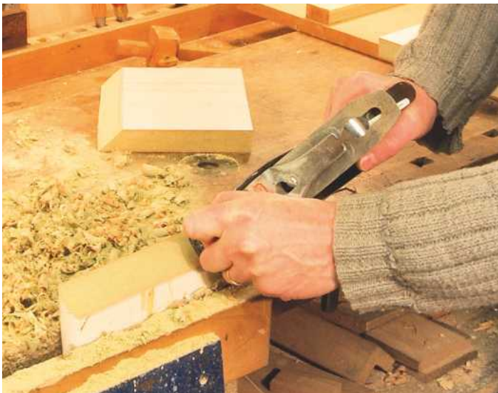
▲ Pic.7 Planing in the sawn mitres for a home-made mitre box. This is MDF which I don't like because of the dust, but for jigs it is perfect because it doesn't warp. Take dust precautions though
